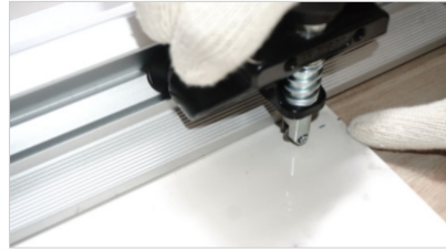
5.1.3 Make sure the wheel is positioned to its place. Press and slide the cutter
