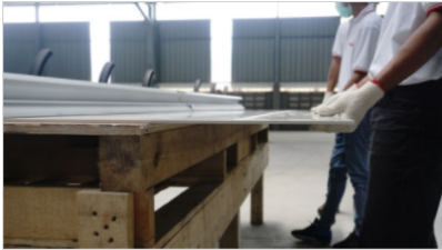
5.1.4 Move the incision line 10cm out of the workbench
