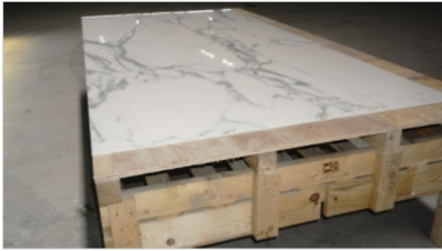
5.1.1 Lay the slab on a stable flat and firm surface
